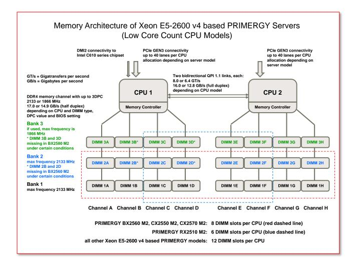
The details about frequencies and bandwidths also take the processor class viewed in the respective diagram into consideration.
