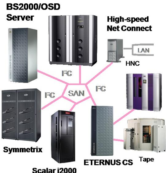
Fibre Channel connects the S servers directly to SAN storage facilities and networks. The FC technology thus permits intelligent implementation and optimal utilization of modern peripheral concepts based on the Storage Area Network model. The advantages are the ability to overcome great distances, a high level of data security, high throughput rates, and standardization of procurement and operations.
