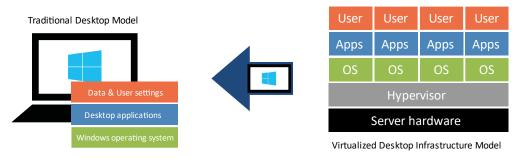
Using hypervisor technology, VDI essentially hosts 'virtual machines' that mimic desktop PC hardware, presenting the Windows operating system to the user with what appears to be dedicated system resources, such as processors, RAM, and storage. VDI comes in two 'flavors':
