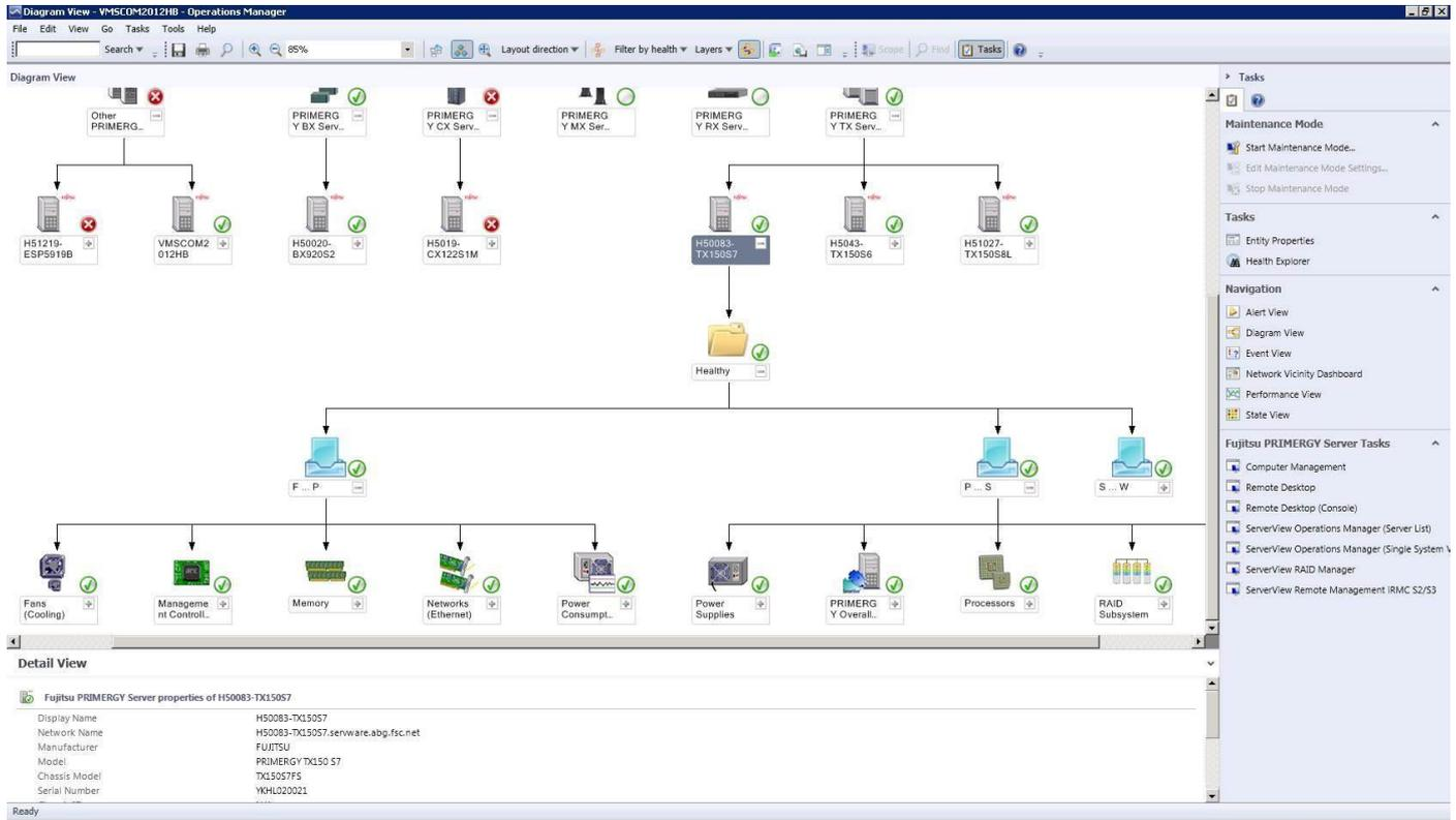
Fig. 2: Microsoft System Center Operations Manager – Diagram View with Fujitsu PRIMERGY servers
