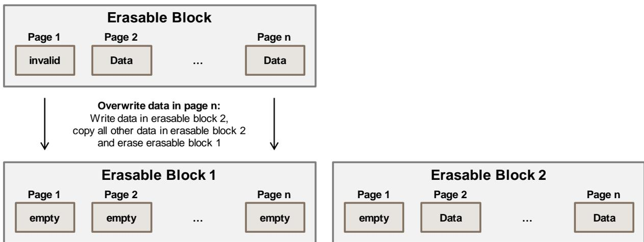
In this way, previously invalid pages are made available again for write jobs. This operation is called **garbage collection**. This ensures uniform wearing of the flash memory cells of pages that are updated (**dynamic wear-leveling**). To also enable the inclusion of flash memory cells of erasable blocks that are not updated in this wearing process, their data is also automatically moved at specific intervals (**static wear-leveling**).
