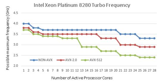
In addition to these general conditions, the quality of the processors also plays a major role for the Turbo Mode performance, particularly with HPC applications. Thus, for example the production variance results in the individual processors of the same type having a different power consumption under the same load.
