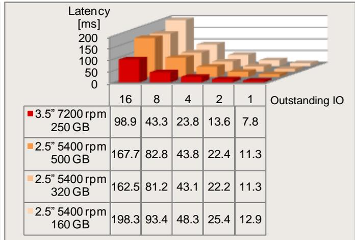
**Standard load profile "Streaming" (sequential access, 100% read, 64 kB block size)**
