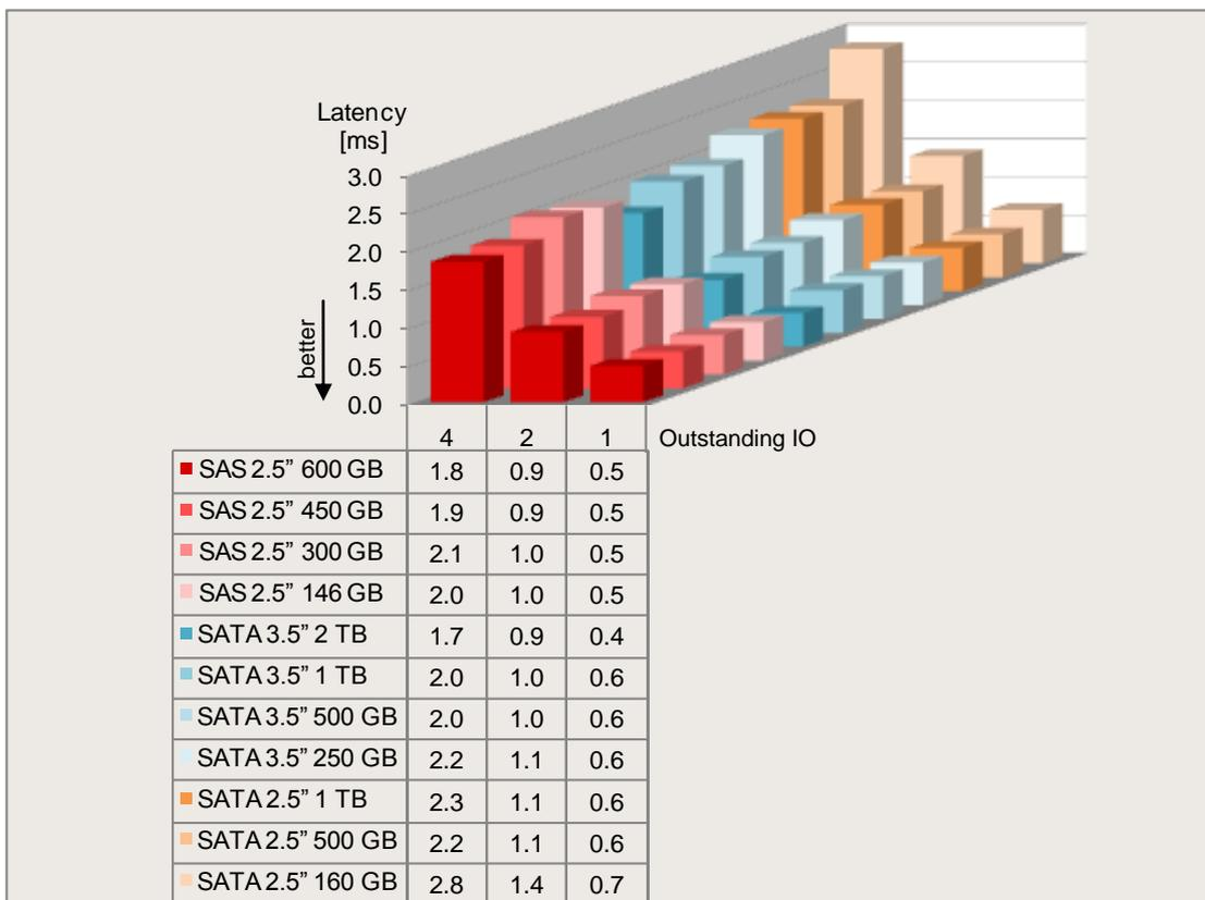
**Standard load profile "Restore" (sequential access, 100% write, 64 kB block size)**
