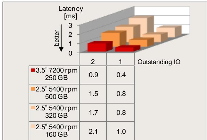
**Standard load profile "Restore" (sequential access, 100% write, 64 kB block size)**
