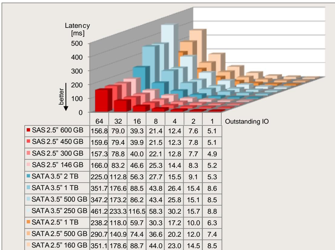
**Standard load profile "Streaming" (sequential access, 100% read, 64 kB block size)**
