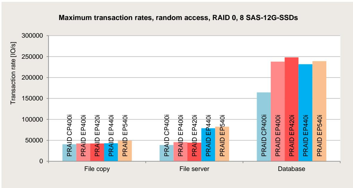
The controllers with cache have a clear advantage for the load profile “Database” (8 kB block size). They also achieve their maximum transaction rate here.
