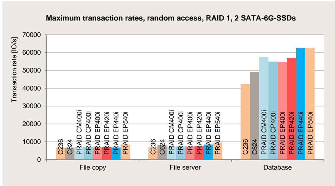
Onboard controllers improve and all controllers achieve similar performance for the standard load profiles “File copy” and “File server” but PCIe controller still has advantages for “Database”.
