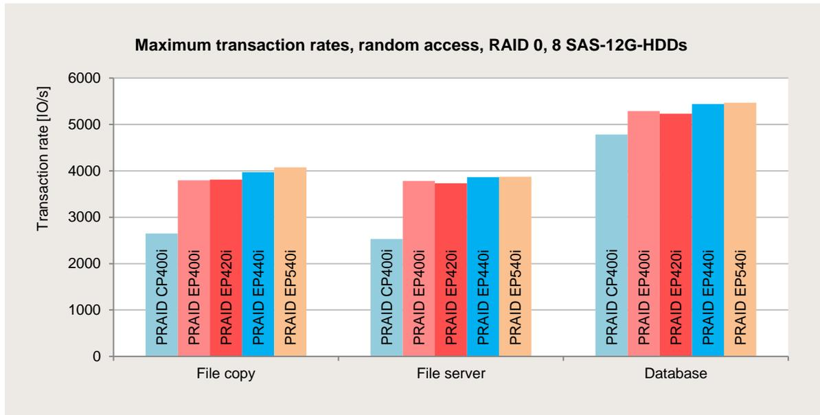
The four right-hand columns in each of the three groups of columns in this diagram represent the four controllers with a cache (PRAID EP400i, PRAID EP420i, PRAID EP440i and PRAID EP540i). The superiority of these two controllers is made possible on the one hand by the controller cache, and on the other hand by the higher default value of the stripe size compared with the PRAID CP400i.
