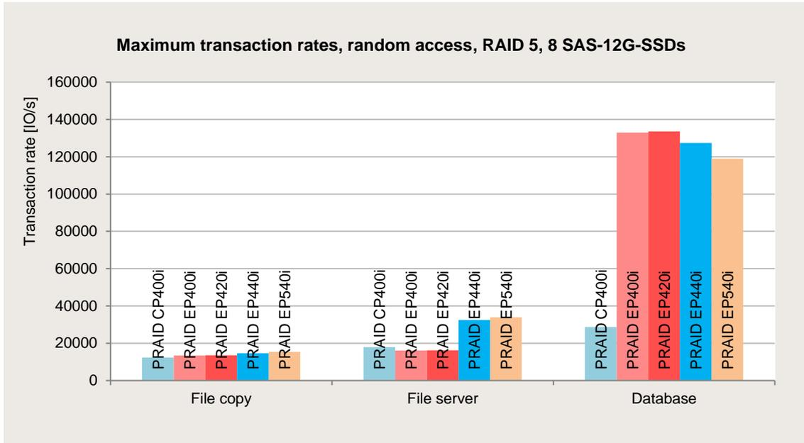
In the case of the load profile with the small blocks (“Database”) the controllers with cache have an advantage here, too.
