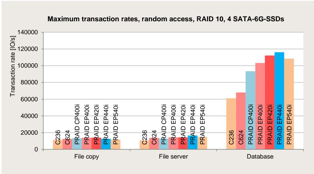
The fact that the transaction rates are higher if the quality of the controller is higher can also be clearly seen here.
