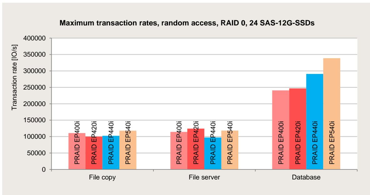
The most important information received here is the very high transaction rate of about 340,000 IO/s that can be achieved for the load profile with a small block size (“Database”). The impact of the FastPath option, which is enabled as standard in the latest controller firmware, is especially apparent for this load profile.
