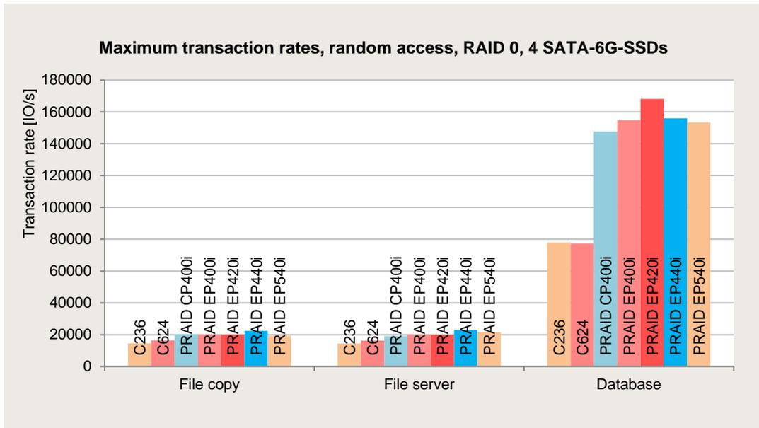
It can be clearly seen that the transaction rates are higher if the quality of the controller is higher.
