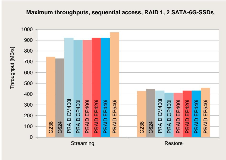
When reading with higher load intensities, the PCIe controllers use both hard disks to a greater extent than the onboard controllers and consequently show a higher maximum throughput.
