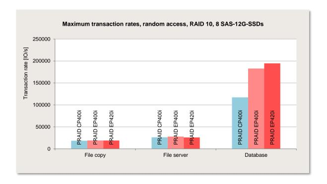
In the case of the load profile with the small blocks ("Database") the controllers with cache have an advantage here, too.
