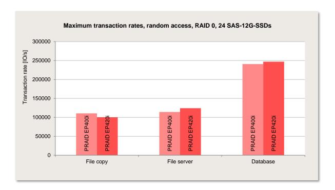
The most important information received here is the very high transaction rate of about 240000 IO/s that can be achieved for the load profile with a small block size ("Database"). The impact of the FastPath option, which is enabled as standard in the latest controller firmware, is especially apparent for this load profile.
