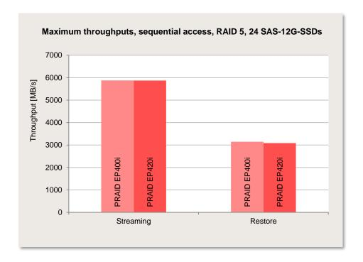
The data throughputs presented here for "Restore" (approx. 3100 MB/s) and "Streaming" (approx. 5900 MB/s) are the limits of the controllers used here for RAID 5.
