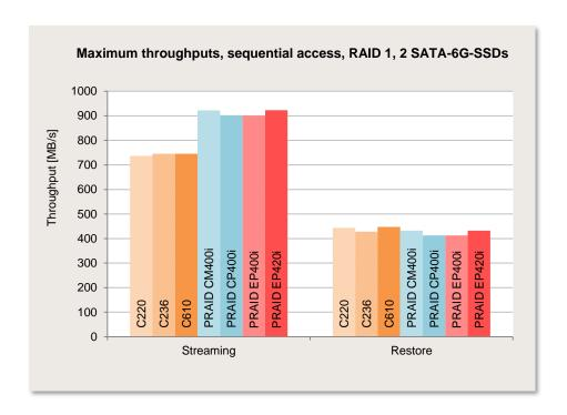
When reading with higher load intensities the PCIe controllers use both hard disks to a greater extent than the onboard controllers and consequently show a higher maximum throughput.
