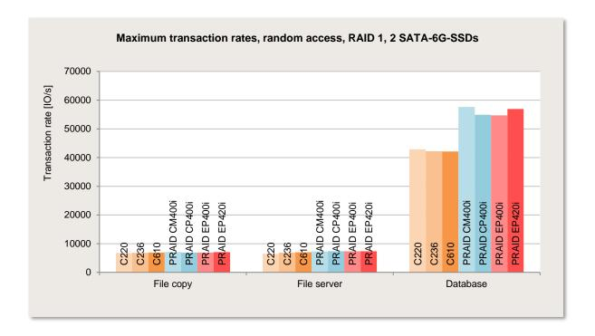
The PCIe controllers provide the highest overall transaction rates here.
