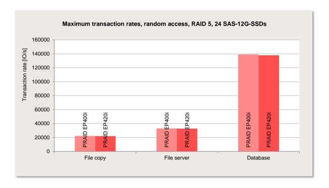
To express this in numbers of SAS-12G-SSDs, it is necessary to have between seven (8 kB block size) and 17 (64 kB block size) fully loaded SAS-12G-SSDs in order to make full use of the possibilities of the PRAID EP400i for RAID 5 - depending on the random load profile. With a smaller SSD load or other SSD types these numbers must be suitably modified.
