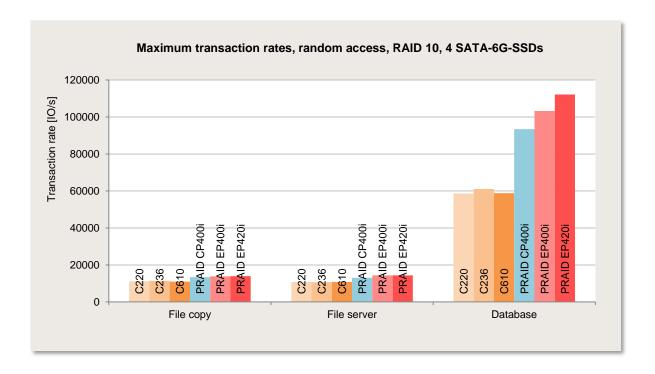
The fact that the transaction rates are higher if the quality of the controller is higher can also be clearly seen here.
