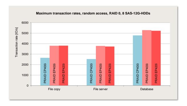
The two right-hand columns in each of the three groups of columns in this diagram represent the two controllers with a cache (PRAID EP400i and PRAID EP420i). The superiority of these two controllers is made possible on the one hand by the controller cache, and on the other hand by the higher default value of the stripe size compared with the PRAID CP400i.
