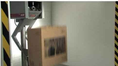
After packaging freefalls from different heights, no damage or cracks must be found on mechanical parts, and the operating system and test program must work normally. Fujitsu tests the thin clients', PCs' and workstations' packaging in three different ways.
