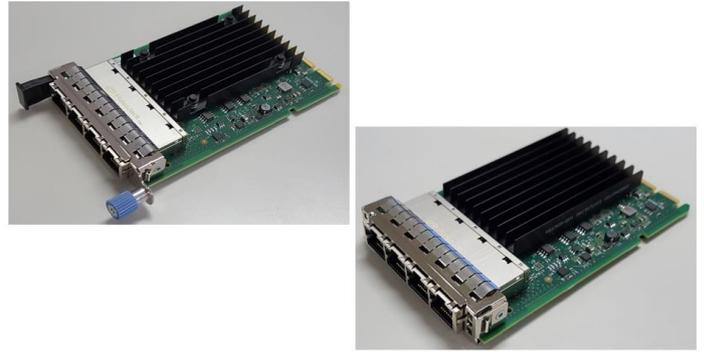
OCP v3 Quad Port 1G BASE-T (Left: Pull tub, Right: Inter Lock)
