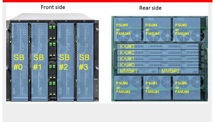
PRIMEQUEST 2000 much reduces cables because components are linked by metal board called mid plane. This means maintenance operations for PRIMEQUEST does not require cabling inside chassis. If taking off and taking on of cables were necessary, power-off of PRIMEQUEST chassis would have been necessary. So, this PRIMEQUEST design helps reduce downtime for maintenance (Figure 16)
