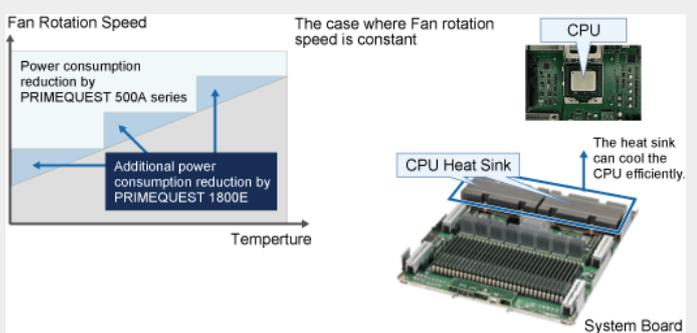
**Figure 11. PRIMEQUEST system board cooling**
