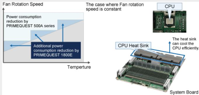
**Figure 11. PRIMEQUEST system board cooling**
