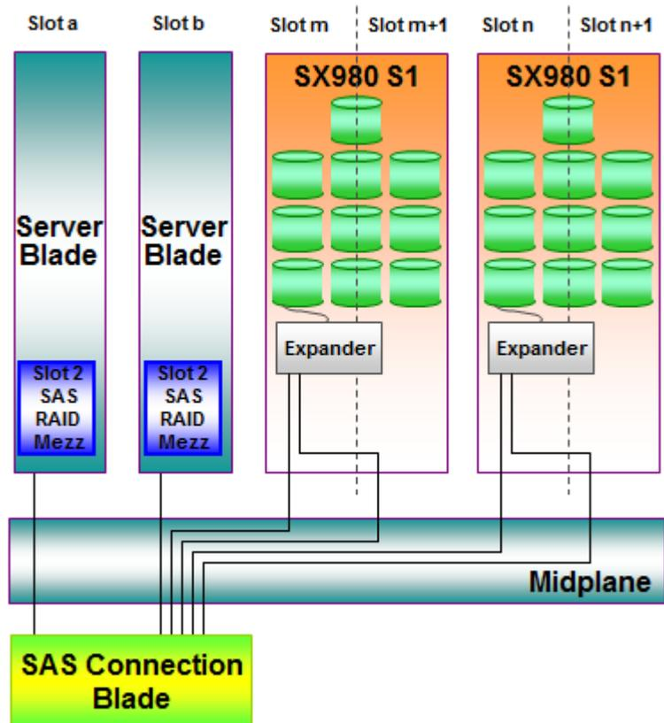
Up to six PRIMERGY SX980 S1 can be plugged into the PRIMERGY BX900 S1 blade server. Up to three PRIMERGY SX980 S1 can be plugged into the PRIMERGY BX400 S1 blade server. Each one occupies two slots in the blade server.
