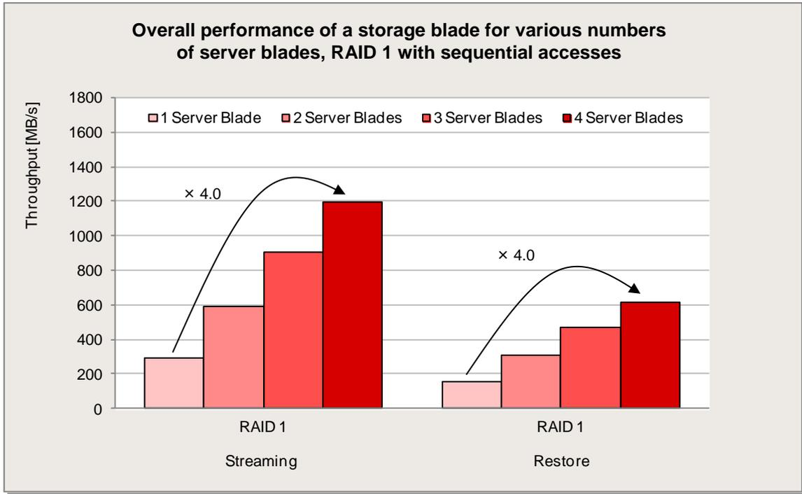
You can also see very clearly here that the overall performance of the PRIMERGY SX980 S1 multiplies at approximately the rate at which the number of RAID arrays increases. Thus, the accesses of several server blades to the same PRIMERGY SX980 S1 storage blade do not appreciably impair each other.
