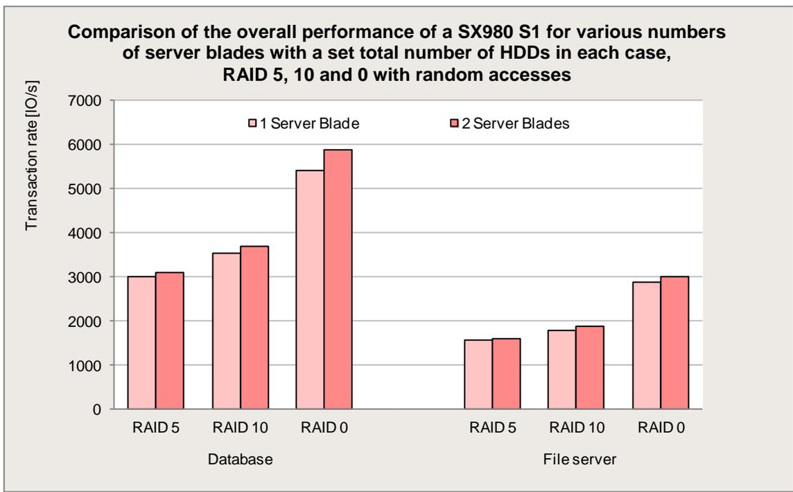
For the random accesses dealt with here it can thus be seen for all three RAID levels that the overall performance increases slightly due to the allocation of the load-generating applications to two server blades instead of to one.
