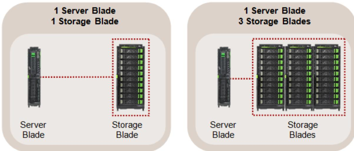
The cases dealt with here are the RAID levels 5, 10 and 0. The number of hard disks per storage blade is constant for each of the three RAID levels. The exact structure of the RAID arrays is described in the following table.
