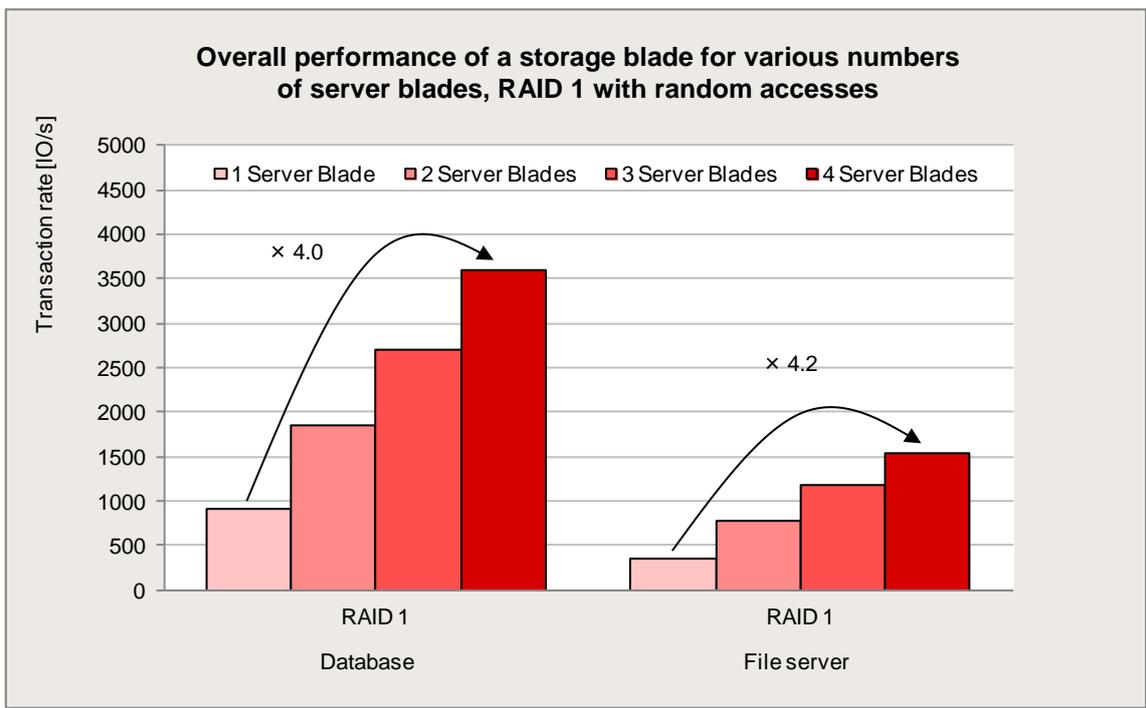
In the diagram you can clearly see that the transaction rates created by several accessing server blades virtually do not impair each other.
