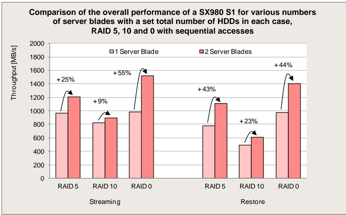
The diagram shows that in the three RAID levels analyzed a PRIMERGY SX980 S1 achieves significantly higher total throughputs for sequential accesses if two server blades, instead of one server blade, access the same total number of hard disks in a storage blade
