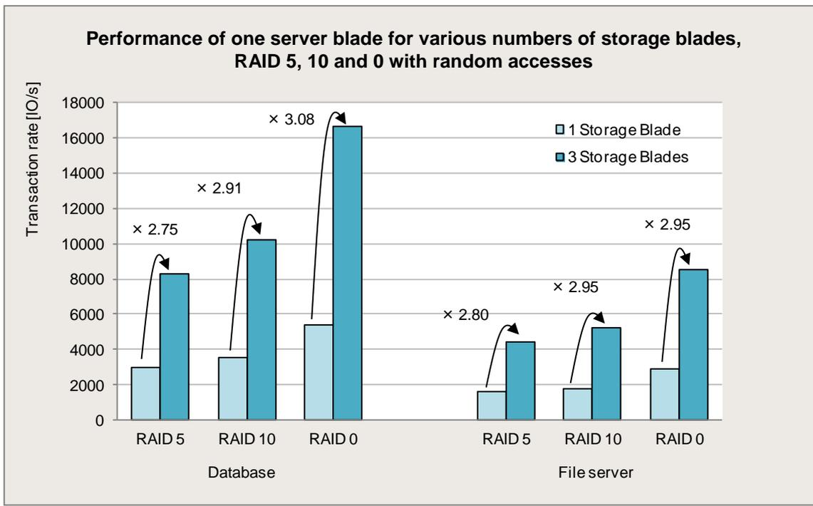
The diagram shows that in all these various cases a server blade with three storage blades achieves approximately three times the transaction rate than with a single storage blade.
