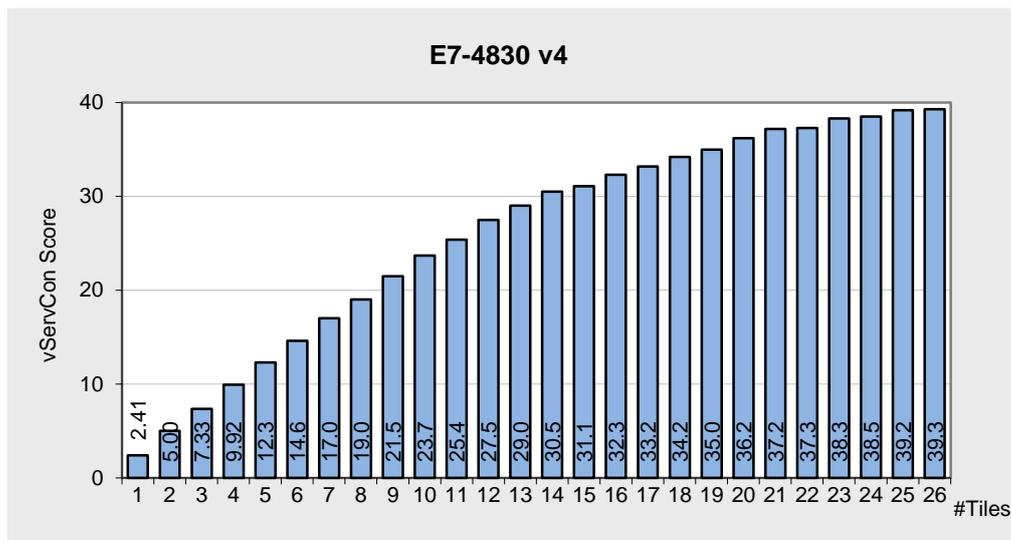
In addition to the increased number of physical cores, Hyper-Threading, which is supported by all Xeon E7 processors, is an additional reason for the high number of VMs that can be operated. As is known, a physical processor core is consequently divided into two logical cores so that the number of cores available for the hypervisor is doubled. This standard feature thus generally increases the virtualization performance of a system.
