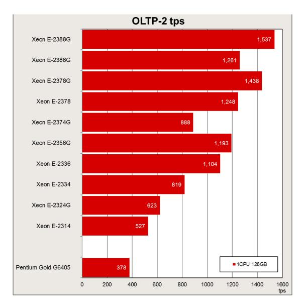
In general, the relatively large performance differences between the processors can be explained by their features. The values scale on the basis of the number of cores, the size of the L3 cache and the CPU clock frequency and as a result of the features of Hyper-Threading and turbo mode, which are available in most processor types. Furthermore, the data transfer rate between processors ("UPI Speed") also determines the performance.
