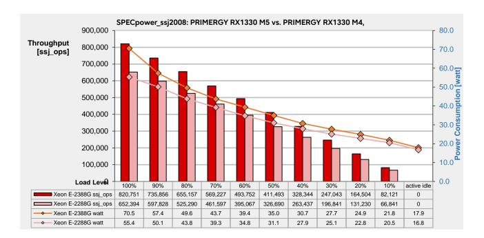
The total average throughput of the PRIMERGY RX1330 M5 is 4,508,248 ssj\_ops, an improvement of 24.6% over the 3,617,215 ssj\_ops of the PRIMERGY RX1330 M4..
