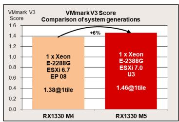
The graph on the left compares the VMmark V3 scores of the PRIMEGY RX1330 M5 and the previous generation PRIMEGY RX1330 M4. The PRIMERGY RX1330 M5 achieved a 6% improvement in score compared to the previous generation PRIMERGY RX1330 M4. This is due to the improved performance of the Intel Xeon E processor and the effective use of the capabilities of the VMware ESXi hypervisor.
