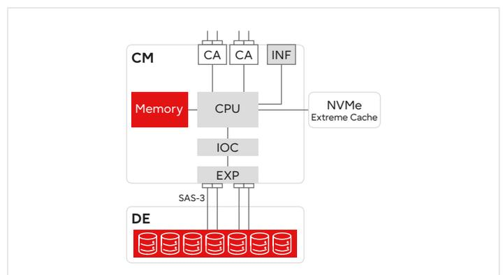
Figure 2: Controller Module (CM)
