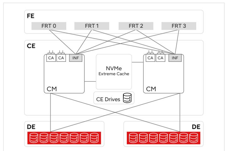
Figure 3: Front-end Routers (FRT) enable PCIe 3.0 high-speed data interchange between the controllers.
