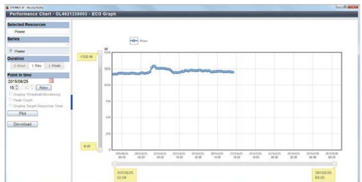
Figure 9: Real-time monitoring of power consumption and temperature with ETERNUS SF helps raise storage administrators' awareness for saving energy.
