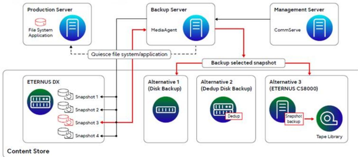
In the setup illustrated above, IntelliSnap supports the snapshot capability of Fujitsu Storage ETERNUS DX hybrid storage systems. The following steps are required:
