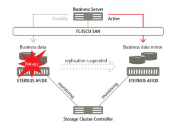
Storage cluster can be deployed in Fibre Channel (FC) and iSCSI environments. Thus organizations can leverage existing skills, because Ethernet is common standard and fast enough for most organizations.
