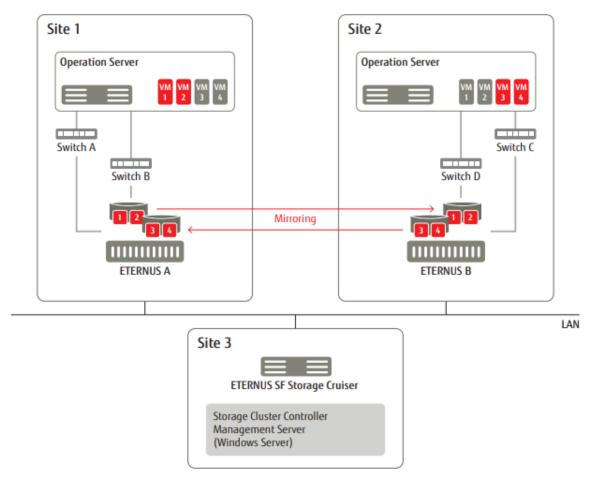
Under normal conditions, VM1 and VM2 at site 1 and VM1 and VM2 at site 2 are connected to the respective ETERNUS AF/DX arrays located at the same site – this is called the active (primary) site. All data is synchronously replicated to the standby (secondary) site, while in this example ETERNUS B is secondary for VM1 and 2 and ETERNUS A is secondary for VM 3 and 4, respectively.
