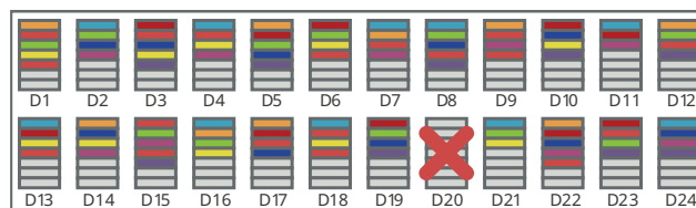
24-drive pool with one drive that has failed
