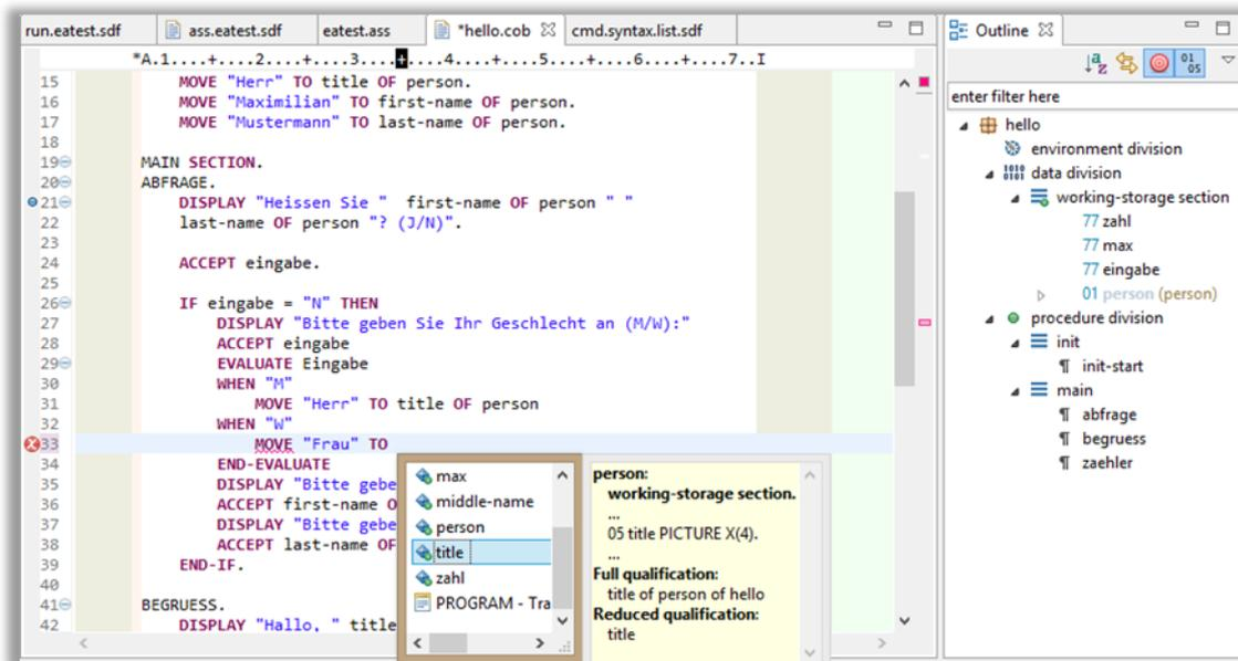
Furthermore, this editor detects a range of typical mistakes while typing and indicates those to the developer by markers similar to spell-checkers of common word processors. The input method (insert/replace) changes automatically depending on the cursor's position. By providing a Java-like Look&Feel this editor especially helps programmers of Java or similar languages to familiarize themselves with COBOL.
