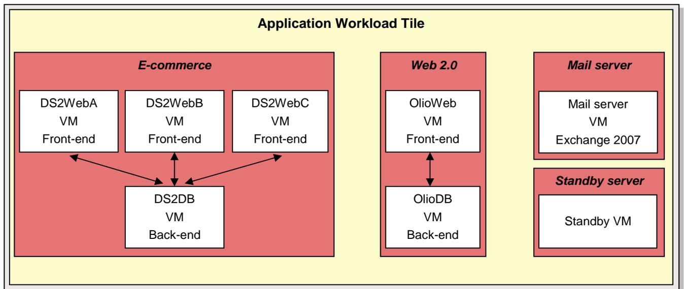
A new feature of VMmark V2 is an infrastructure component, which is present once for every two hosts. It measures the efficiency levels of data center consolidation through VM Cloning and Deployment, vMotion and Storage vMotion. The Load Balancing capacity of the data center is also used (DRS, Distributed Resource Scheduler).
