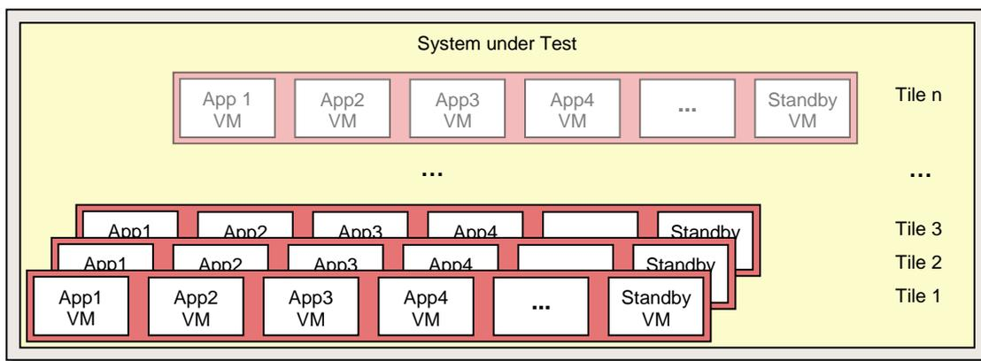
An application is executed in each virtual machine where the applications are put under stress via established benchmarks. If necessary, there may also be further infrastructure components. All the individual results are then suitably summarized in one overall result. This score is an indication for the performance capability of a virtualized environment.
