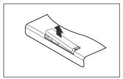
Slide the protective rubber cover of the SIM card slot in the direction of the arrow.
