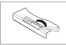
Open the protective rubber cover over the SIM card slot.
