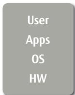
In traditional PC architecture, the life cycles of the hardware, operating system, applications, and user profiles are closely interconnected.
