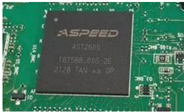
iRMC S6 – integrated Remote Management Controller
