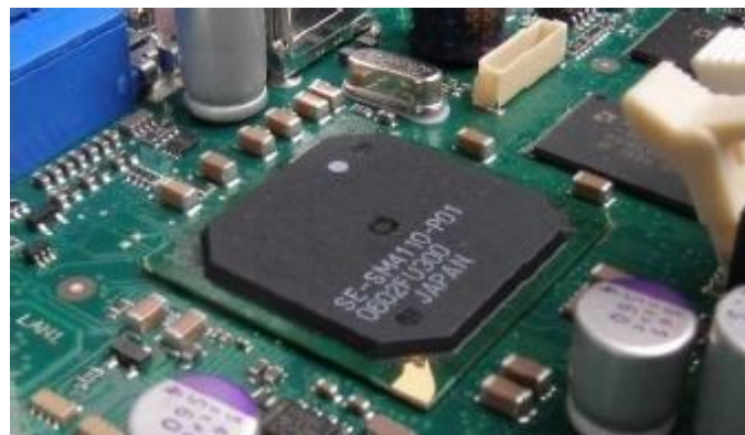
iRMC S3 – integrated Remote Management Controller
