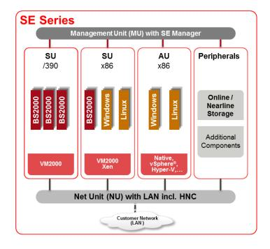
Beside the net units data and management network, a connection of the customer network to the SE server is possible via LAN controllers inside HNC, SU x86 or AU. This enables fast data connections with 10 Gbit/s directly into the customer network without the10 Gbit/s NU extension for SE servers.
