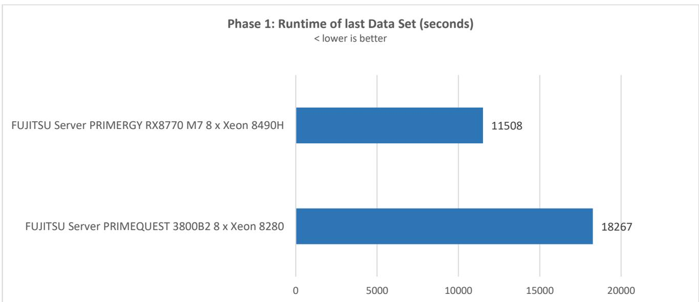
Phase 1 is the data load phase. It is a combination of CPU- and IO-intensive load.
