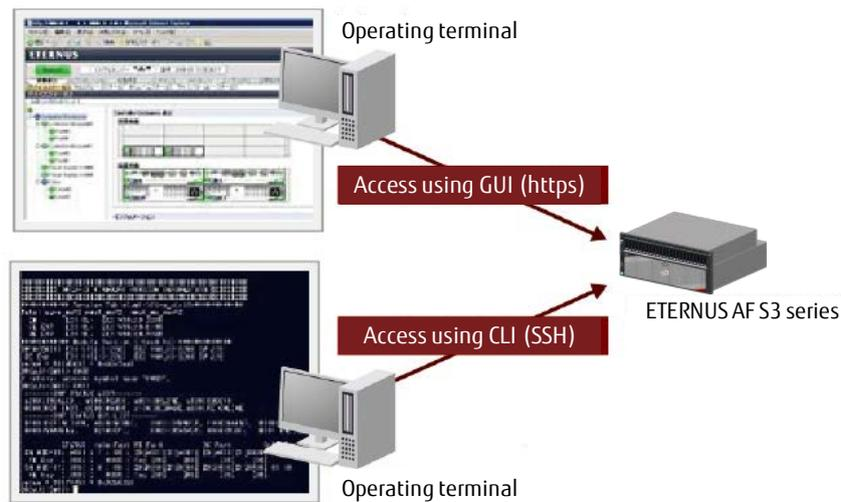
Figure 5-5 Strengthened Security with SSL/SSH
