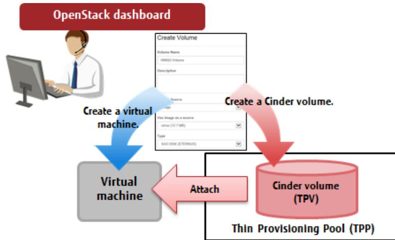
Figure 5-8 Operation of the OpenStack Dashboard
