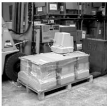
First place an unfolded carton on an empty pallet covered by a layer of bubble wrap to avoid any scratches on the monitors. Place the monitors face down with the bases facing inwards, wrapping each layer in stretch foil to prevent slipping. Cover the first layer with another unfolded carton and bubble wrap.
