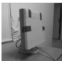
TFT monitors are extremely sensitive to pressure and require particular care when packaging. Ideally you should use the original boxes, but as if these are not available it is recommended to use similar sized boxes. Attach a piece of Styrofoam (the size of the whole screen, not just the viewable area) to the front of the TFT so that any eventual pressure is spread equally over the TFT casing. Fill any gaps in the carton (including between the casing and the cardboard) with adequate bubble wrap.
