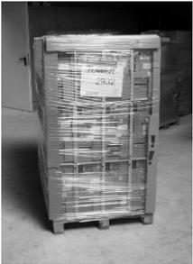
Not all printers are suitable for packing in layers unless they are already adequately boxed. Due to the weight of the printers, it may not make sense to pack them on top of each other.
