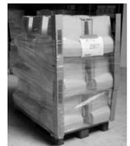
**It is important** that all monitors are covered, if necessary using two unfolded cartons and sufficient bubble wrap, as this forms the base for the next layer of monitors. It is preferable to use the same quantity of monitors for each level so that the layers are loaded to an equal height. Repeat the process for the third layer.
