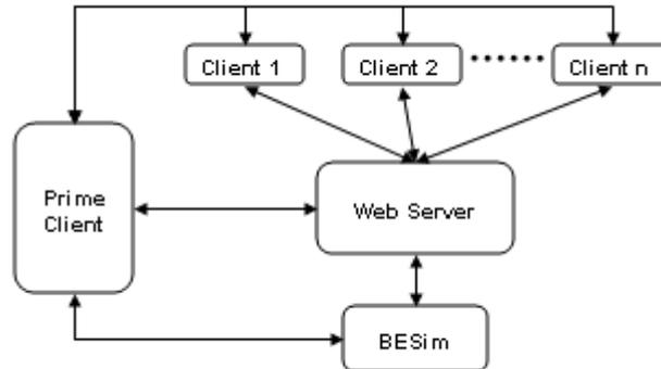
**Figure 1: Logical components in SPECweb2005**
