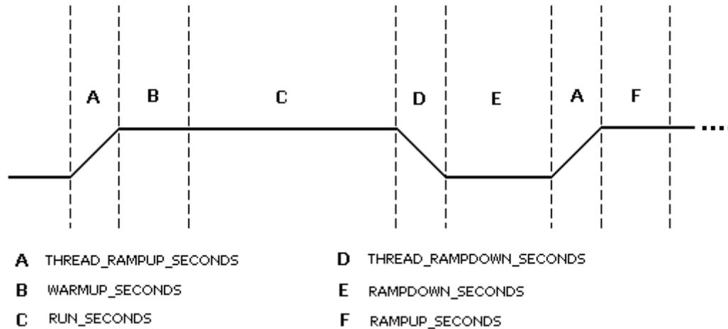
**Figure 2: SPECweb2005 test phases**
