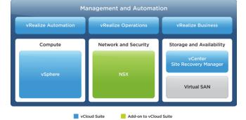
Note: Cloud management platform components of vCloud Suite, including vRealize Automation, Operations, and Business, are specifically designed for use with vSphere environments. vCloud Suite can be extended to hybrid cloud with vRealize Suite.
